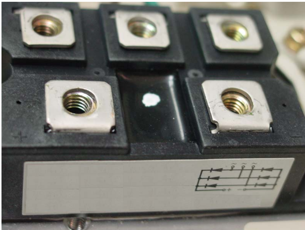
Figure 21: Diagram of rectifier module
