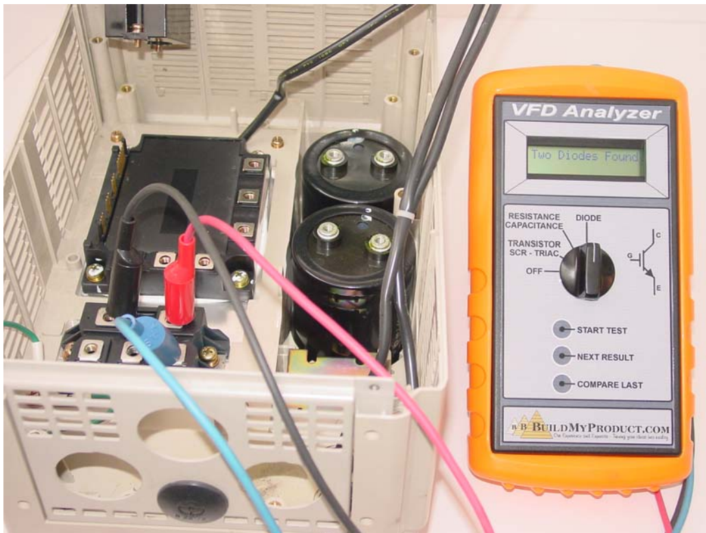
Figure 23: Verifying third pair in rectifier module
