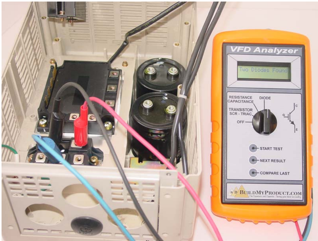
Figure 22: Verifying second pair in rectifier module
