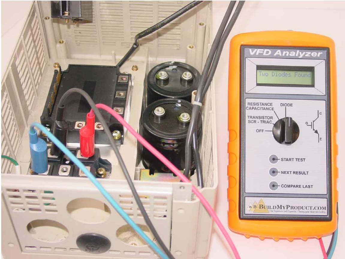
Figure 19: Verifying first pair in rectifier module
